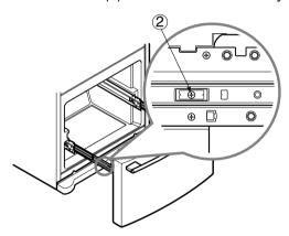
Lift the top of door to unhook door supports from rail system. Lift door up to remove.
